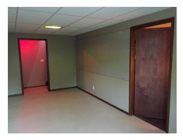
After transforming the old libraryoffice space into a modern control room, we continued the remodeling of the Z-dome with the hallway. The ceiling tiles were refurbished, the walls were repaired and painted. The concrete floor was resurfaced with an epoxy paint. An addition of a trim molding made the floor work complete.
