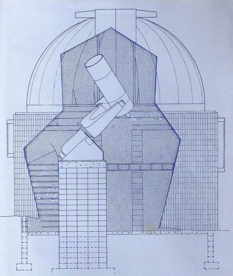
telescope when it's not in use, has two floors, each 24 feet square. The upper floor accommodates the moving telescope, its mounting, the control panel, and people; while the ground floor will have support equipment, meeting space, and educational exhibits.
