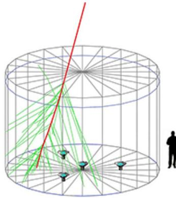
*Each corrugated steel tank in HAWC is 7.3 meters across and 4.5 meters deep. It contains a bladder filled with ultrapure water. At the base are four photomultiplier tubes. This diagram shows a charged particle (red line) passing through a tank and emitting Cherenkov radiation (green lines). Credit: Image created by Brian Baughman of the University of Maryland and Segev Benzvi of the University of Wisconsin.*
